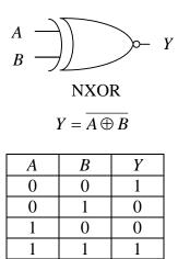
The output is a "1" when A and B are of the same value. The output is "0" when A and B are of different values. It is said the Y equals A exclusive nor'd with B. Note that it is incorrect to say Y equals not A exclusive
