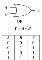
The output is a "1" when A or B or both are "1". Otherwise, the output is a "0". It is said the Y equals A or B. The electrical circuit below illustrates the concept.
