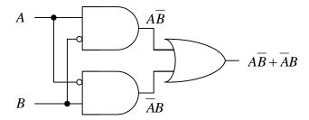
The output is a "1" when A and B are of different values. The output is "0" when A and B are of the same value. It is said the Y equals A exclusive or'd with B.
