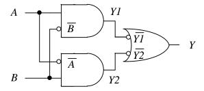
It should be noted that the circle indicates that the input is complemented and the complemented input is shown inside the gate for convenience. First generate the equation for Y1,  $Y1 = A\bar{B}$ . Second, generate the equation for Y2,  $Y2 = \bar{A}B$ . Third, generate the equation for Y,  $Y = \bar{Y}1 + \bar{Y}2$ . Finally, substitute the equations for Y1 and Y2,  $Y = \bar{A}\bar{B} + \bar{A}\bar{B}$ .
